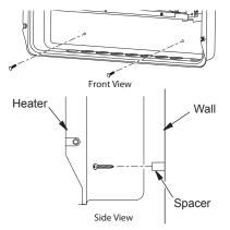
Figure 12 - Installing Bottom Mounting Screws
